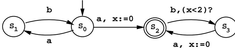
Figure 5: Timed Büchi automaton accepting  $L_{\text{crt}}$
