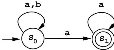
Figure 1: Büchi automaton accepting  $(a + b)^*a^\omega$
