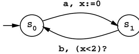
Figure 3: Example of a timed transition table
