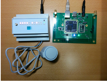
Fig. 5. Seluxit devices: gateway (top right), relay box (top left), valve (bottom)
