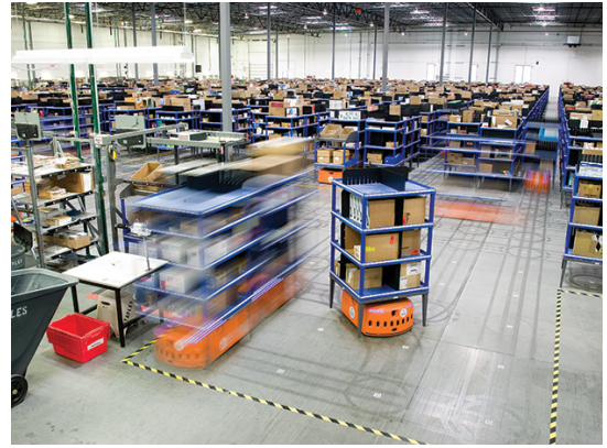
Fig. 1. Amazon Robotics, or formerly known as Kiva System. Picture from Guizzo (2008)
