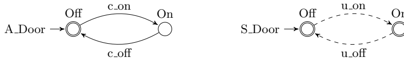
Fig. 2. Examples of two plant models, with an actuator of a door and a sensor of a door. Concentric circles indicate marked locations. Solid arrows indicate controllable events while dashed arrows indicate uncontrollable events.
