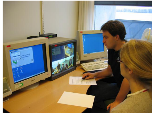
Figure 5. Observation room: relayed screen signal from test PC and video signals from cameras in the subject room-
