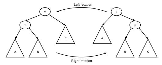
Figure 4: Left and Right Rotations
