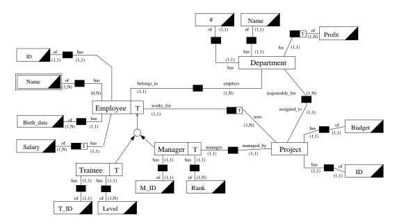
Figure 2: An ERT Diagram Describing a Company Database
