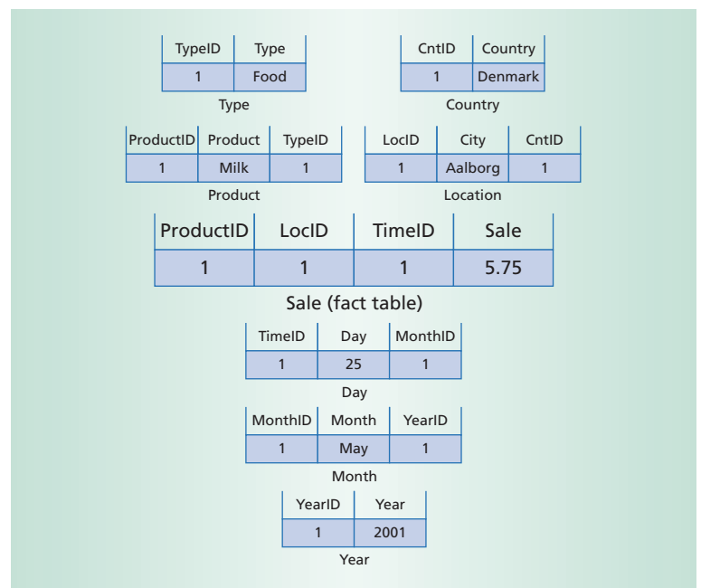
Figure 4. Snowflake schema for sample sales cube. Information from different levels in a dimension is stored in different dimension tables—for example, product names and product types are stored in the Product and Type dimension tables, respectively.
