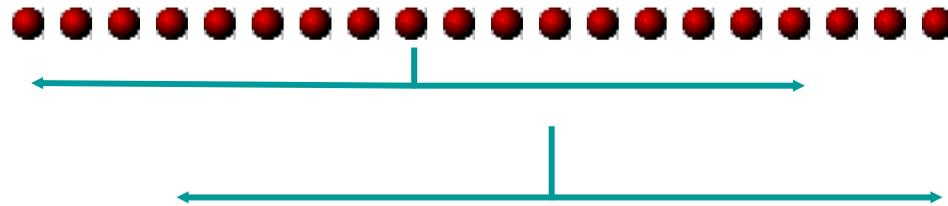
*Each node maintains IP addresses of the nodes with the  $L$  numerically closest larger and smaller node IDs, respectively.*
