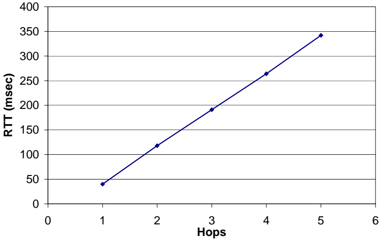
Fig. 4. Round trip times for various route lengths. Note that one hop measures the time for a message between the Host PC and base station device.
