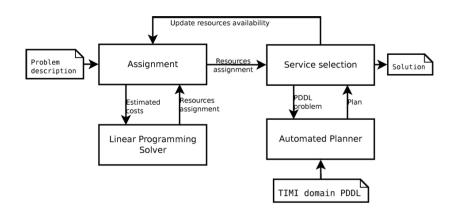
Fig. 4. Workflow of the TIMIPLAN top level algorithm.
