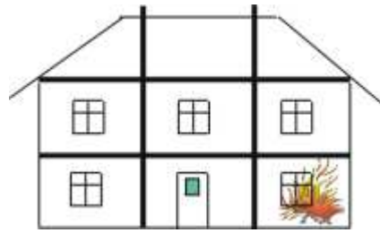
Figure 11.3 A house - with firewalls - on fire. The fire is not likely to spread to other apartments because of the solid firewalls.
